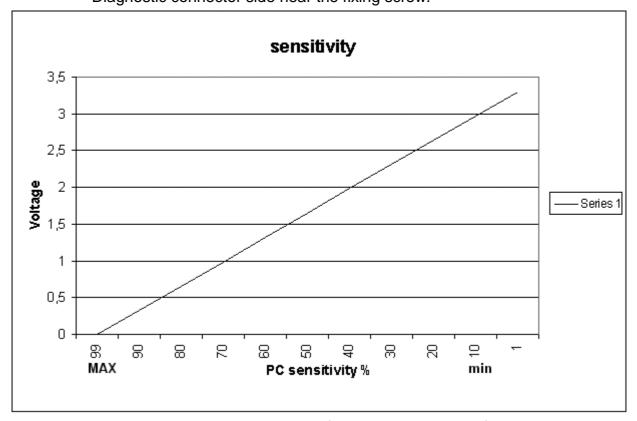
Remember that selecting at half the voltage value of the trimmer to obtain average sensitivity. In fact, the voltage value indicates the system's level of sensitivity. 3.3Volts indicates the minimum sensitivity. At this setting, the system will detect the intrusion of large objects.
