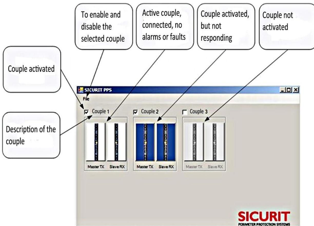
Check the box with symbol √ the couples present (active) and used in the system.
