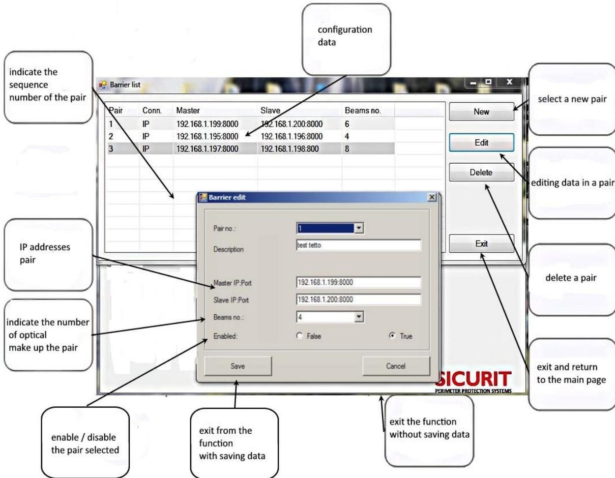
**The IP address must be associated with the communication port 8000.
