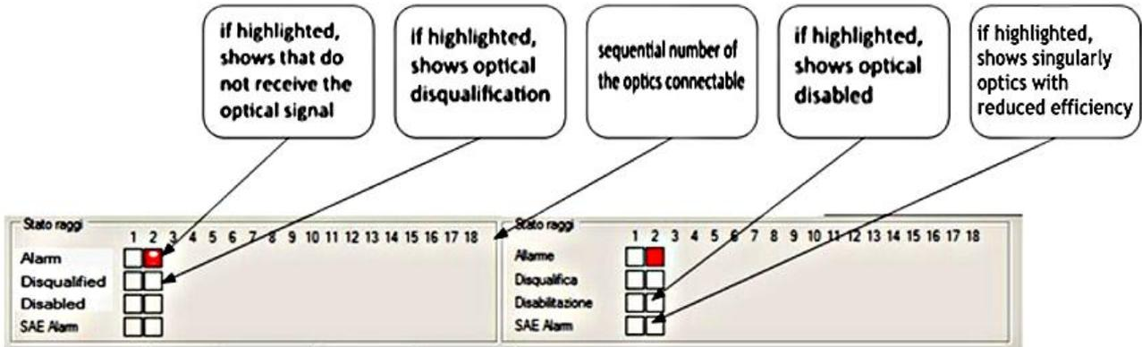
Selecting the window "Intrusion analysis" will open the page of MW analysis intrusion alarm, useful for setting the correct values of sensitivity and delay detected by simulations crossings. Selecting the window "Beam will open the page settings and diagnostics of each optical element connected to the system. Selecting the window "Alarm config" will open the settings page of the individual response times for each optical receiver and alarm scenarios in groups of optical.
