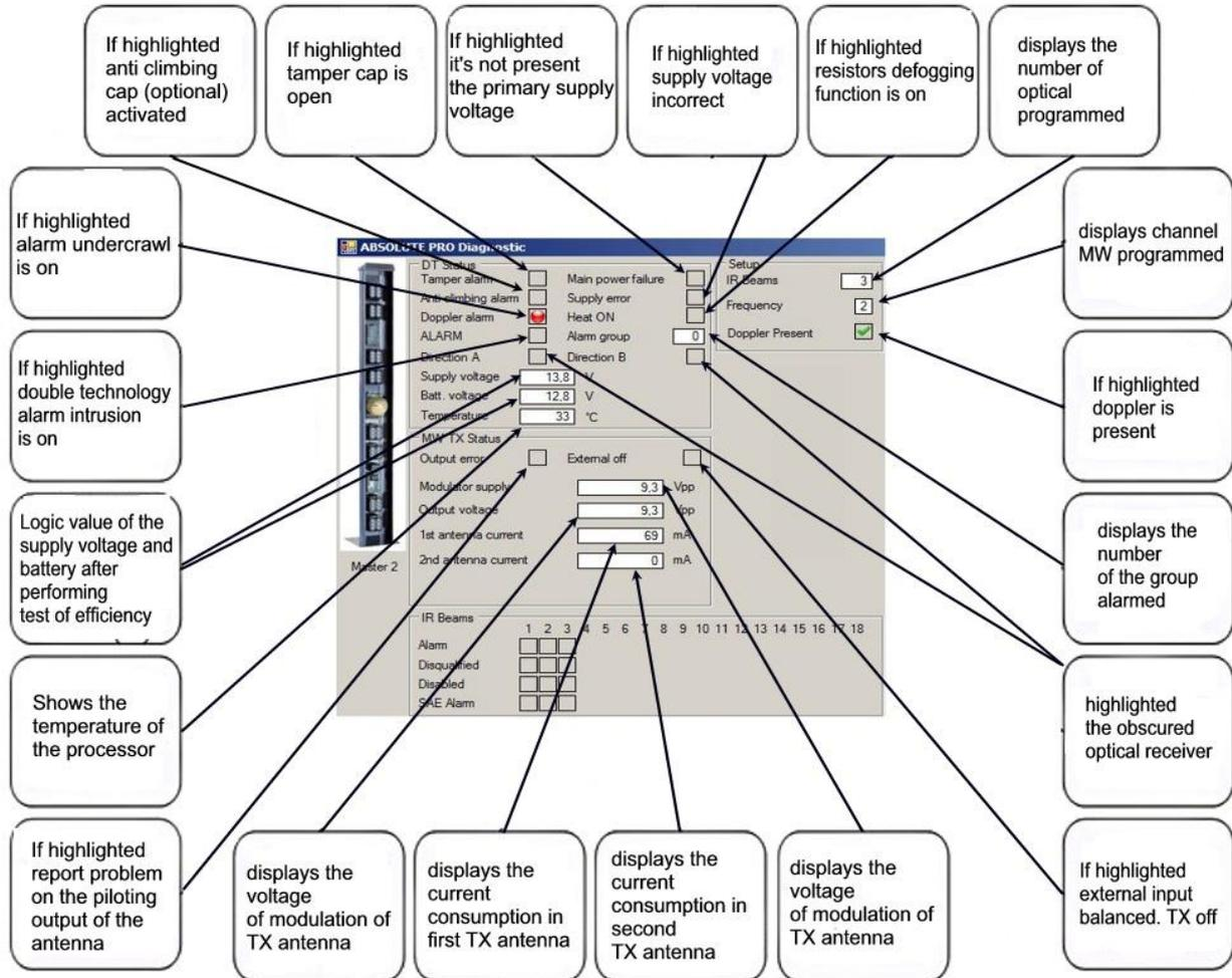
The supply voltage square box will indicate the battery voltage value (last test value) when the Main power error box will be signed.
