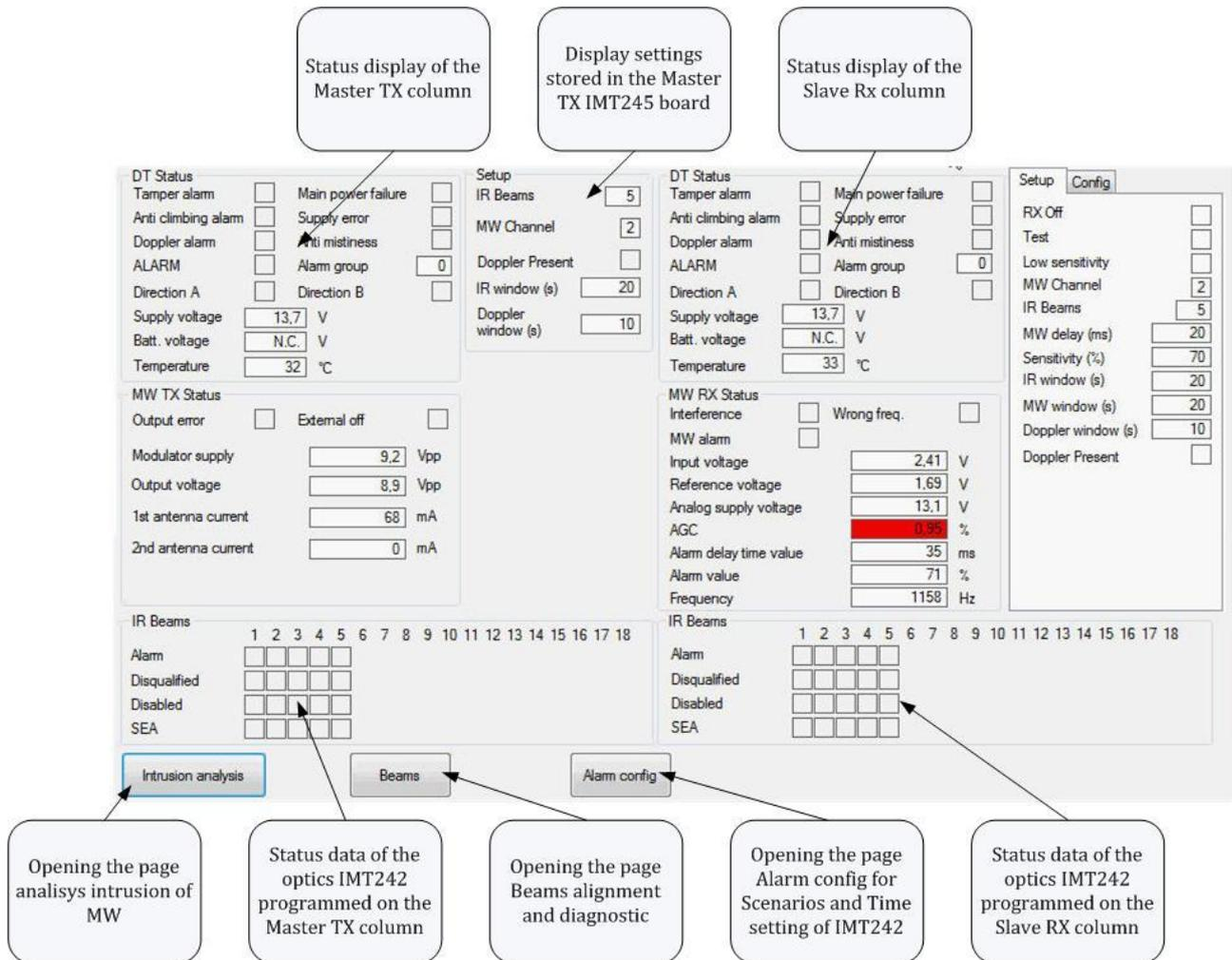
In the top panel the general parameters of the system status of the connected system will be shown.
