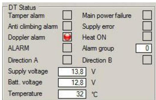
When the primary supply voltage is not present, the box is highlighted with the color green power for correct voltages, yellow for voltages out of range and red for incorrect voltages. The value in volts of the battery box indicates the last value measured during the test day. The test battery efficiency is performed after 10 seconds from the power system and daily.
