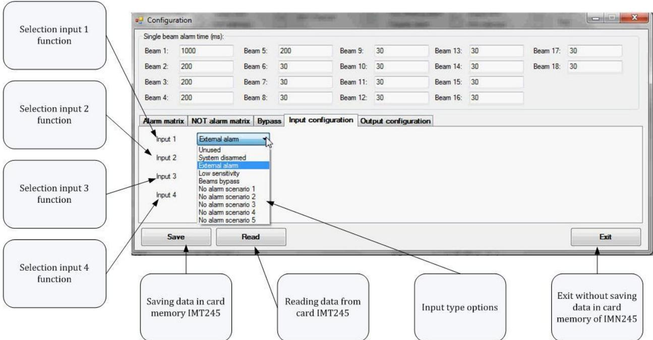
Each input can be associated to the BYPASS or to NO ALARM scenario number (from 1 to 5 scenario).
